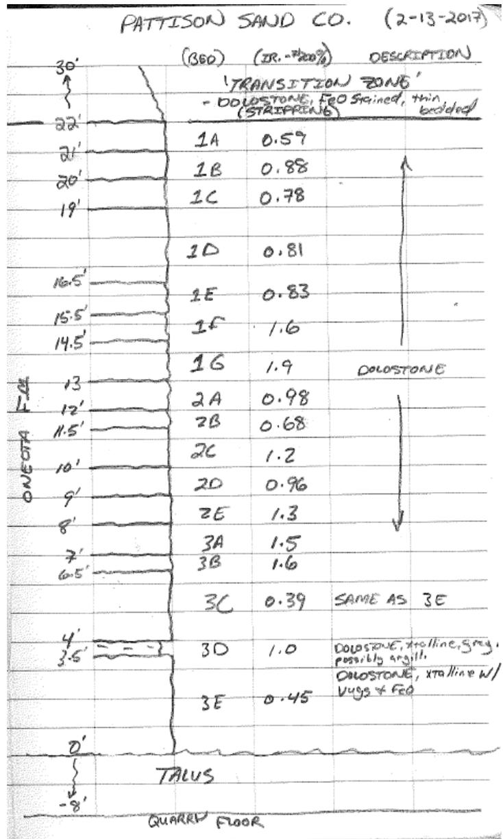
Fig. 4: Scan from field notebook showing delineated beds, bedding plane elevations (see quarry tape in Figure 2), insoluble residue results and bed descriptions (where acquirable).
