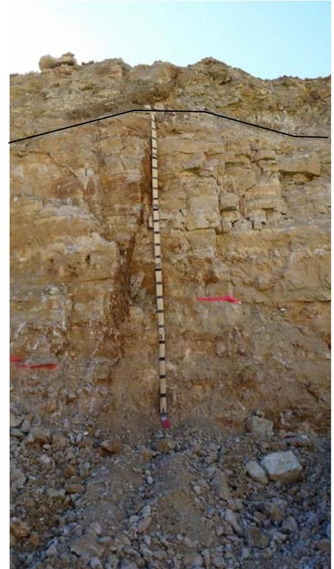
Fig. 2: Photo of portion of production ledge showing fresh dolostone and upper, weathered dolostone stripping ledge (separated by black line)
